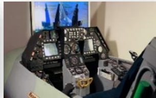
F-16 A/B Avionics Software dev. HIL hybrid lab and simulators
